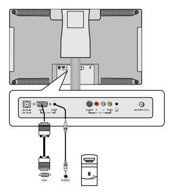
After connection, turn on the unit and the PC and then press the INPUT button to shift to VGA mode.
